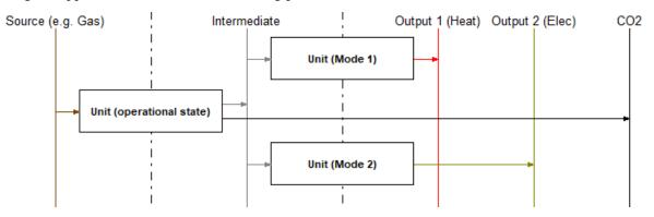
Here the vertical lines represent the commodities and the rectangle are processes. The arrows indicate in- and output commodities of the processes. In the case shown the power plant 'Unit' would be able to operate between a state where only 'Output 1' comes out and a state where only 'Output 2' comes out. The two extreme cases can, however, also be chosen as combinations of both outputs already.
