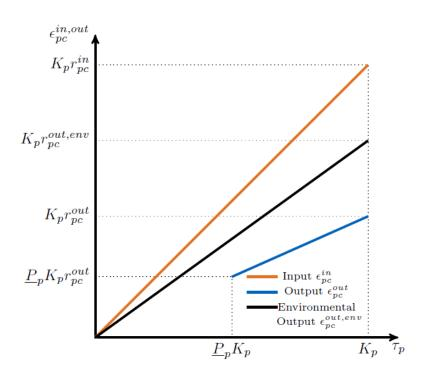
The following graphic illustrates a process with the on/off feature and part load behavior:
