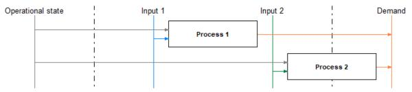
Here the vertical lines represent the commodities and the rectangle are processes. The arrows indicate in- and output commodities of the processes.
