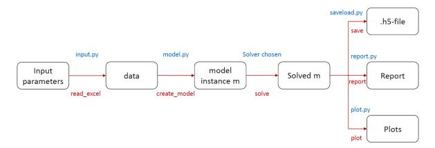
'urbs' uses a modular structure to build and execute the optimization and to automatically generate the results. All scripts are placed in the folder 'urbs'. In subfolder 'features' constraint expressions for the mathematical model are defined. These will not be discussed here and only the highest level functions will be discussed. The scripts used for these are the following (in alphabetical order):
