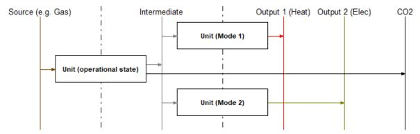
Here the vertical lines represent the commodities and the rectangle are processes. The arrows indicate in- and output commodities of the processes. In the case shown the power plant 'Unit' would be able to operate between a state where only 'Output 1' comes out and a state where only 'Output 2' comes out. The two extreme cases can, however, also be chosen as combinations of both outputs already.
